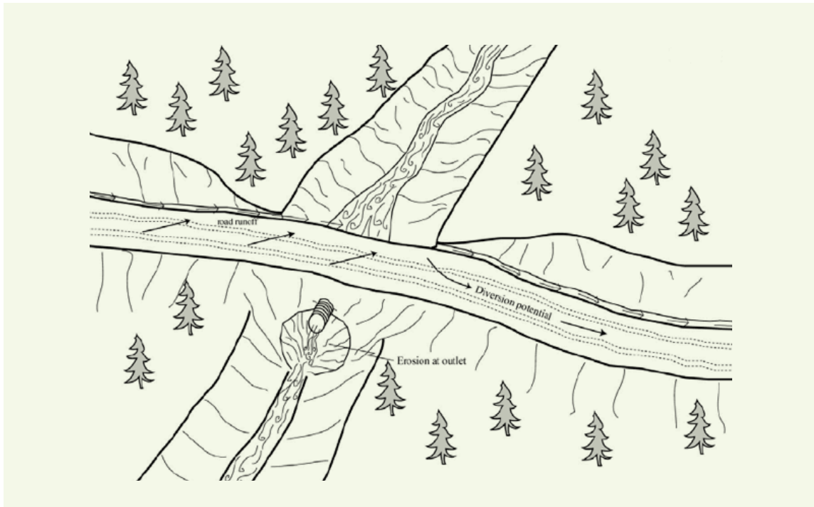
FIGURE 6. Diagram illustrating diversion potential at a watercourse crossing (from DFG 2006).
