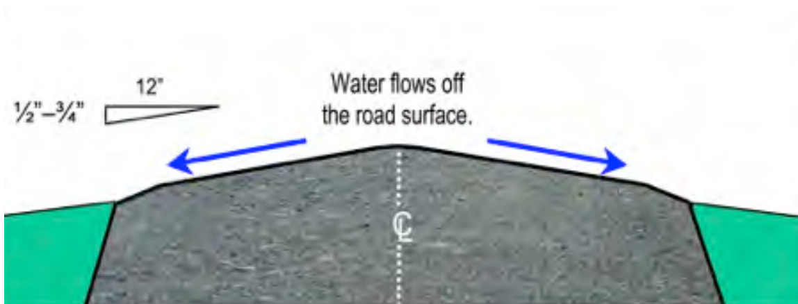
FIGURE 31A. Centerline crown with proper cross-slope for an unpaved road. Road drainage flows without obstruction off the road surface into surrounding vegetation. Note the slight grade increase at the road shoulder to encourage off-road drainage (Center for Dirt and Gravel Road Studies, 2005).
