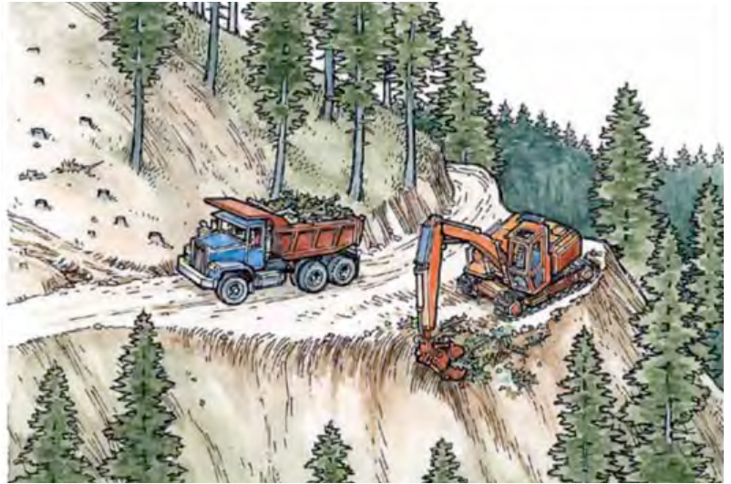
FIGURE 211. Unstable landing fill excavation. Oversteepened fill is removed from the landing edge and endhailed off-site to a stable location (Adams and Storm, 2011).
