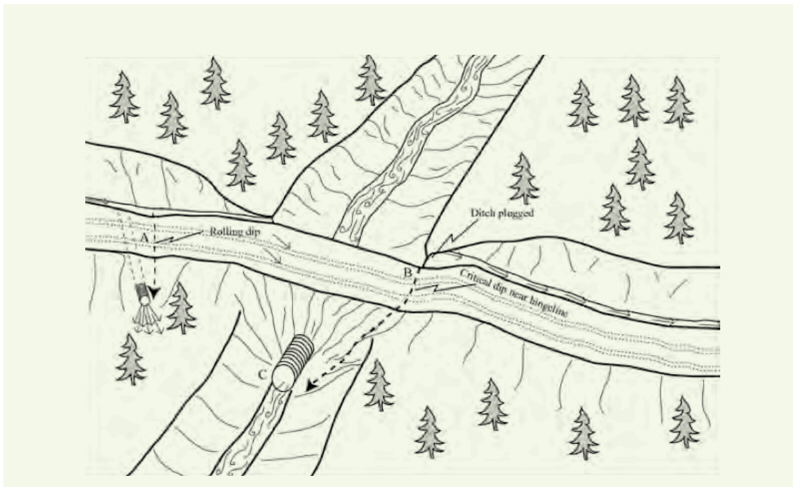
FIGURE 6. Diagram illustrating diversion potential at a watercourse crossing (from DFG 2006).
