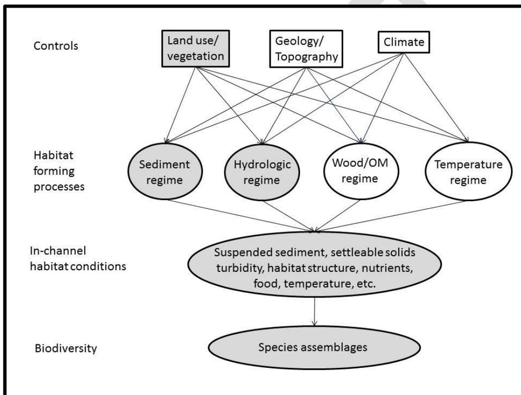
**Figure 1.** A simplified schematic diagram representing “ecological performance” for a riverine aquatic ecosystem. Shaded boxes represent elements of ecological performance potentially addressed directly or indirectly through a Road Rules effectiveness monitoring study. OM stands for organic material (modified from Beechie and Bolton, 1999).
