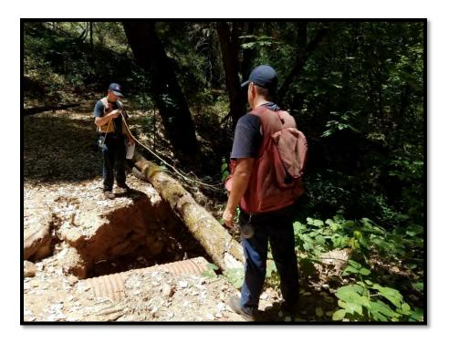
Figure 53. Overtopped culvert delivering >10 cubic yards of sediment to a Class II watercourse in the Sierra area
