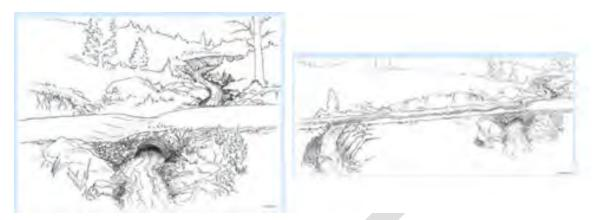
Figure 5: No potential for diversion (Left), and potential for diversion (Right) (Images from Furnis et al., 1997)
