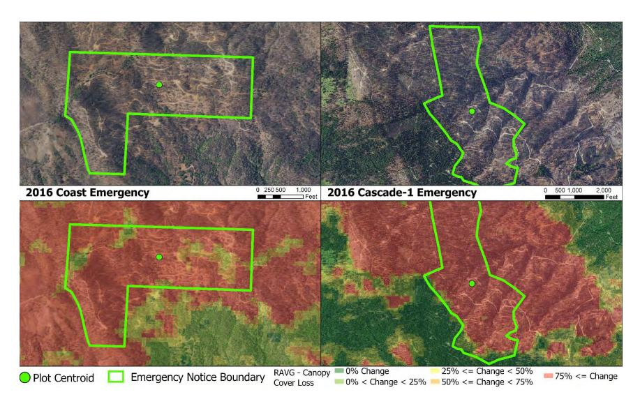
Figure 69. ESRI ArcGIS basemap imagery showing post-salvage harvesting extent (top), and initial assessment RAVG data for the Coast and Cascade-1 Emergencies (bottom).
