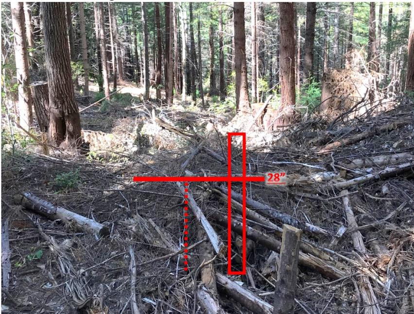
Figure 32: Example of harvest slash depth measurement; from the soil surface to the highest point where slash sticks up, is the slash depth.
