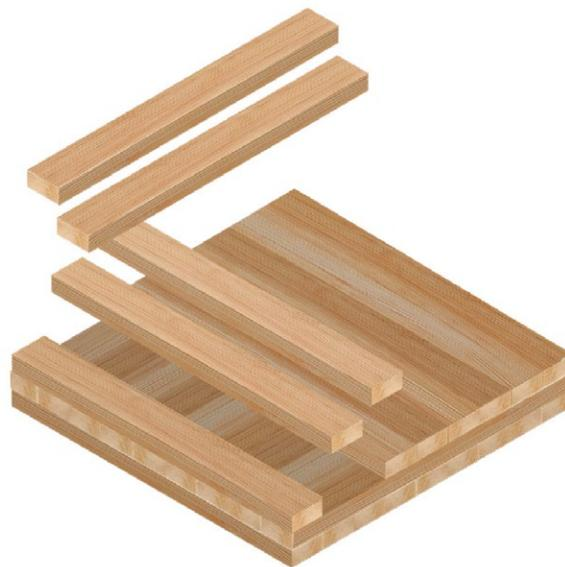
Figure 2. Cross-laminated timber layers. Image from the 2021 Mass Timber Design Manual, courtesy of WoodWorks and ThinkWood ([info.thinkwood.com/masstimberdesignmanual](http://info.thinkwood.com/masstimberdesignmanual))
