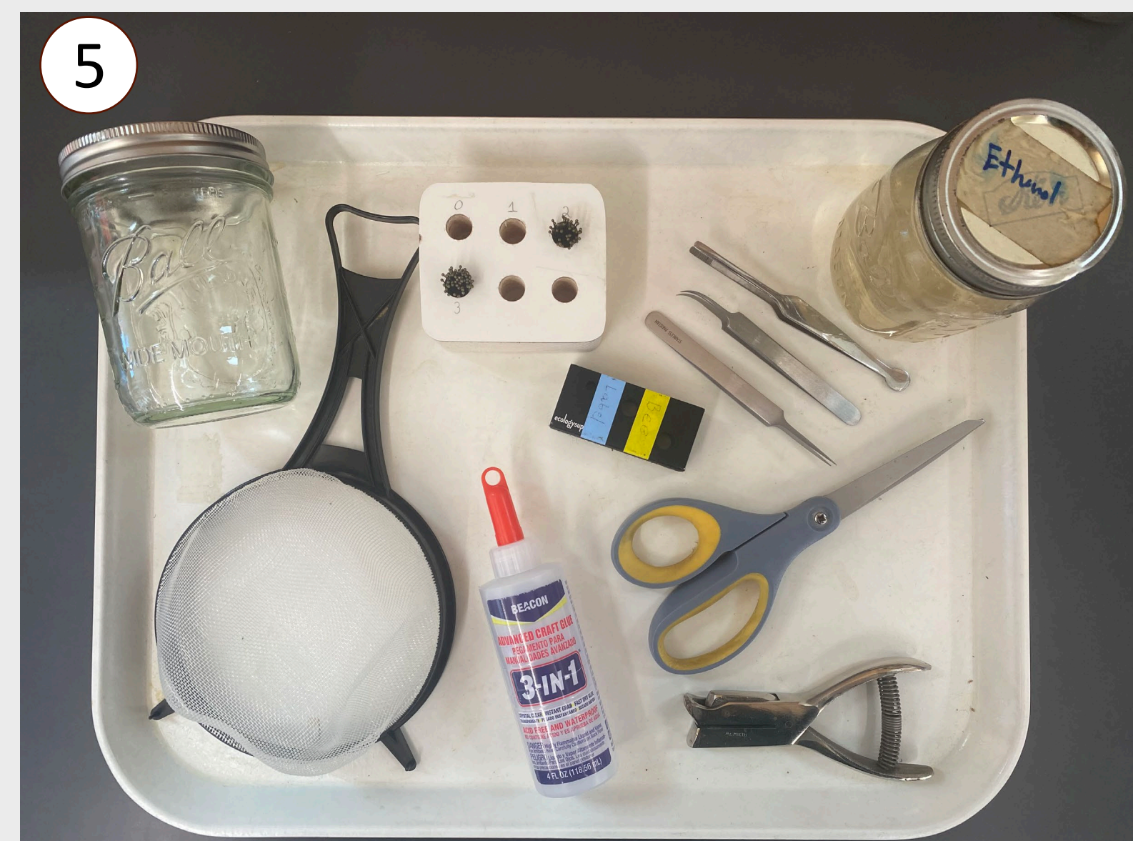
Tools necessary for pinning bees include jar with mesh lid, strainer, pins(assorted sizes), glue, pinning block, forceps, scissors, ethanol, blow dryer.
