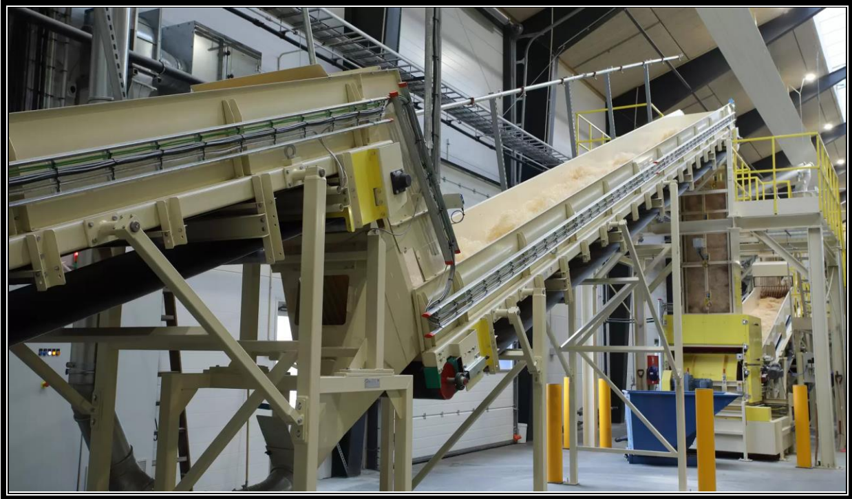
Figure 2.11 – Wood Wool Feeding and Dosing System Ahead of the Station Where Wood Wool is Mixed with Cement and Accelerator
