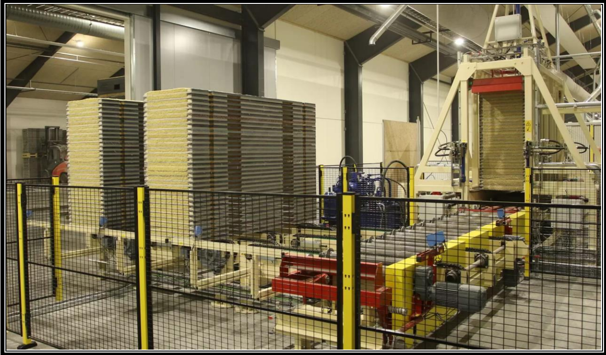
Figure 2.15 – After First Setting Panels are Demolded in Preparation for Second Setting, Which Takes About 10 - 12 Days
