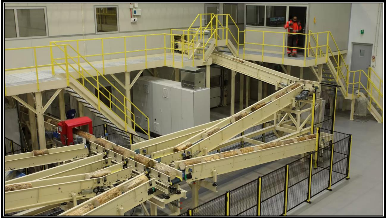
Figure 2.11 – Wood Wool Feeding and Dosing System Ahead of the Station Where Wood Wool is Mixed with Cement and Accelerator
