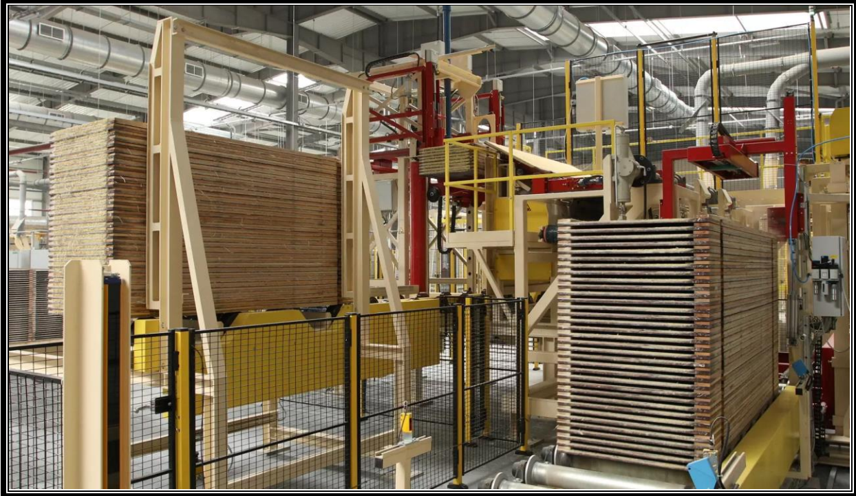
Figure 2.15 – After First Setting Panels are Demolded in Preparation for Second Setting, Which Takes About 10 - 12 Days
