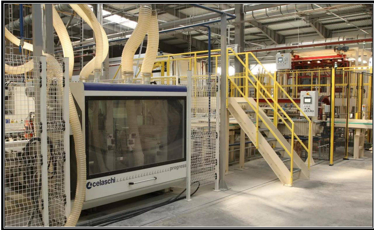
Figure 2.16 – After Second Setting Panels Are Cut, Profiled, Trimmed to Final Dimensions Using CNC Machines, In Final State (not shown) Finished Panels are Packaged for Shipment to Customer
