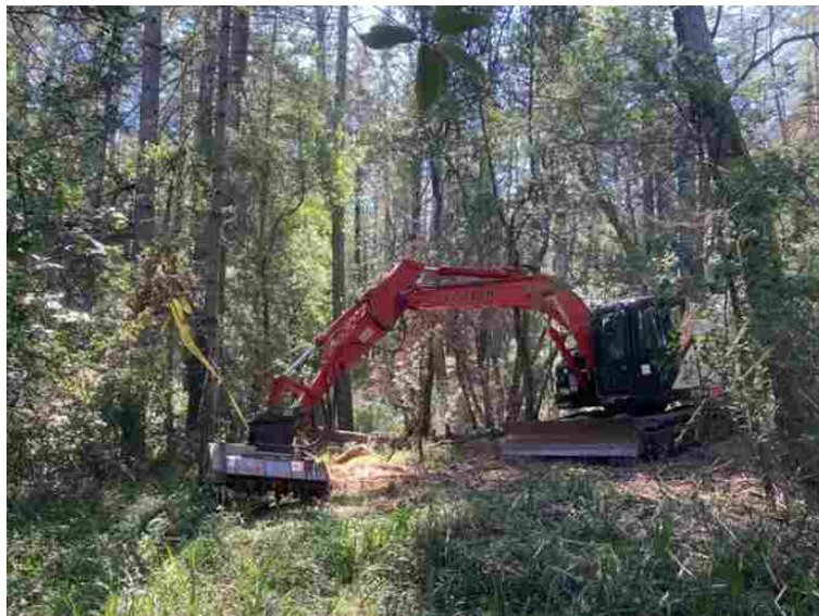
Figure 10: Example of Mechanized Equipment – Link-Belt 145 x 4 excavator with masticating head attachment.
