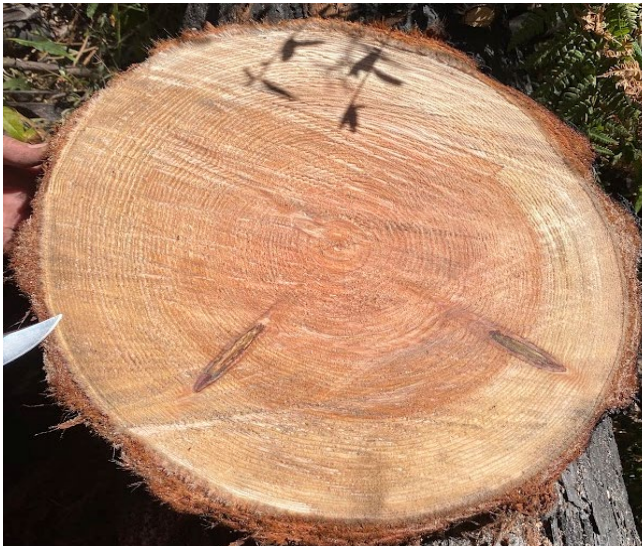
1 st Log small end – No 2020 Damage, yellowing sapwood
