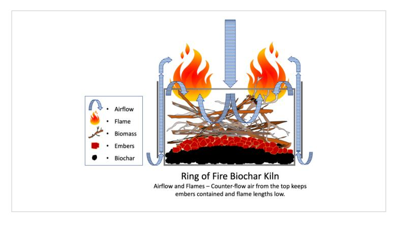
**Figure 1: Schematic showing air flow, flame characteristics, and char accumulation in the Ring of Fire Kiln.** Counterflow combustion air pulls the smoke into the hot zone, where it burns up. Air flowing up through the annular gap between the main kiln body and the heat shield provides pre-heated combustion air to the kiln, further increasing combustion efficiency. Please click here to view a larger version of this figure.
