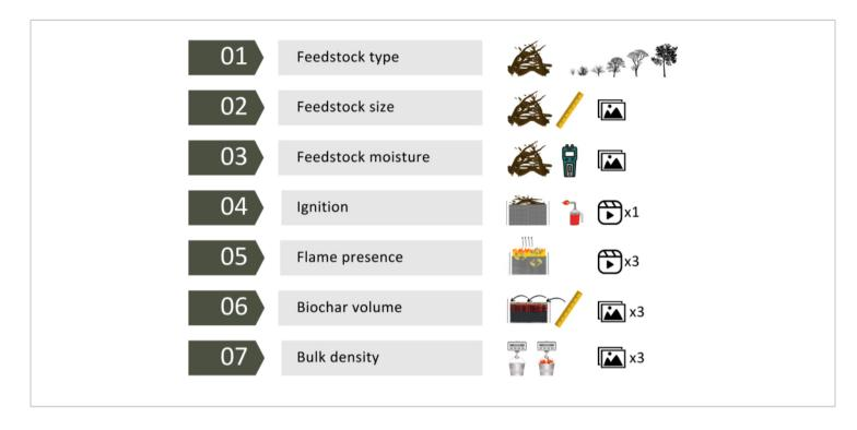
**Figure 2: Infographic showing the process verification points.** The process verification points for a typical batch of biochar made in the Ring of Fire kiln. Please click here to view a larger version of this figure.
