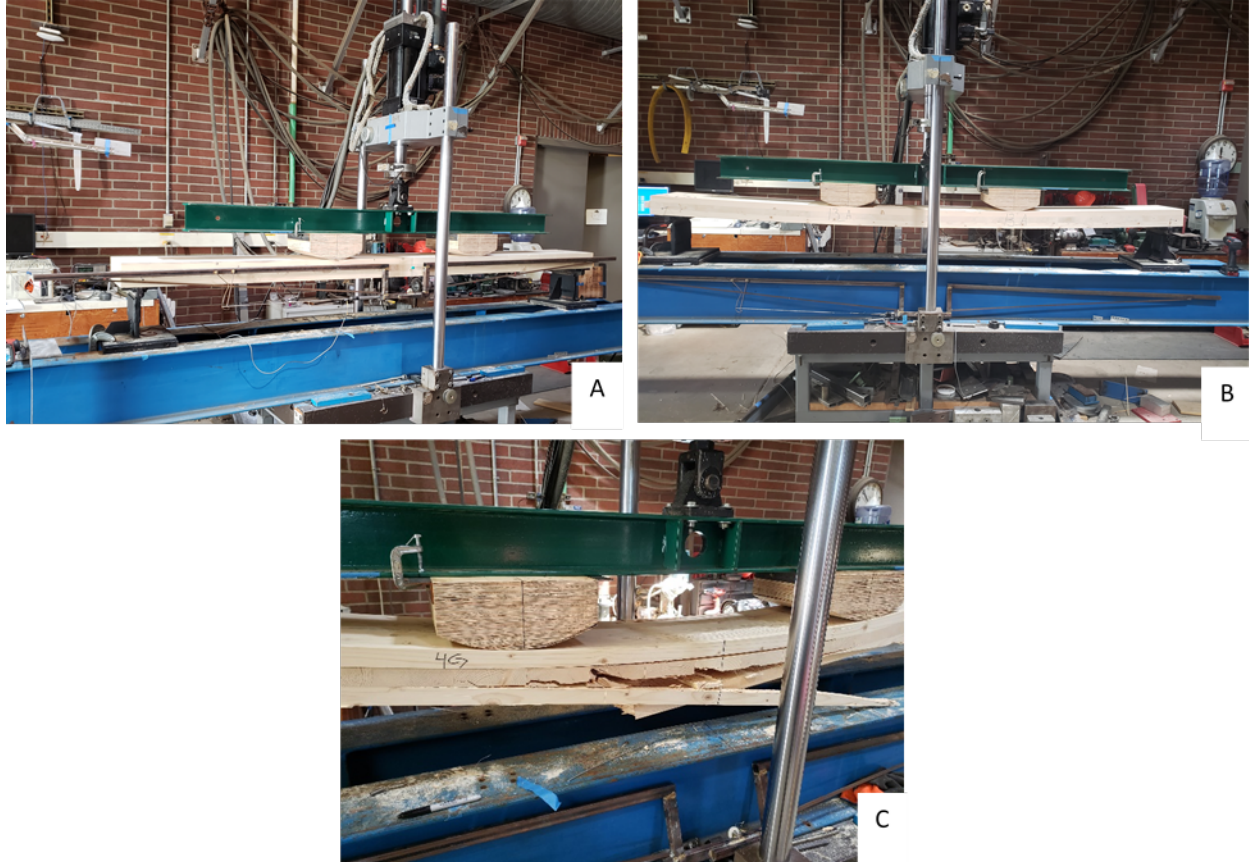
Figure 13: (A) Test Specimen, (B) Test specimen after bridge is removed, and (C) Tension failure of Specimen.
