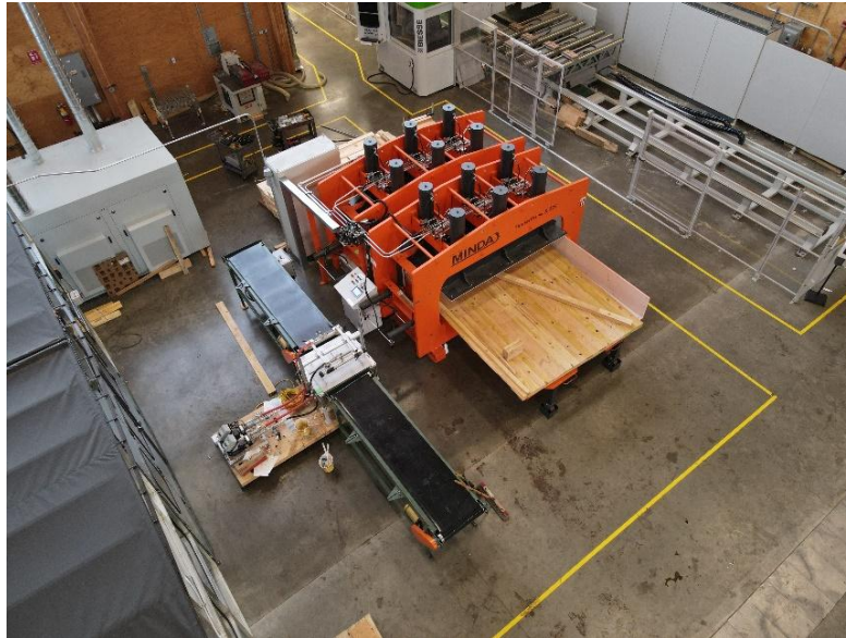
Figure 6: Apquip resin applicator and Minda press
