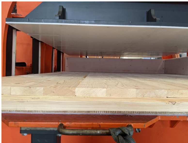
Figure 7: CLT panel immediately after pressing
