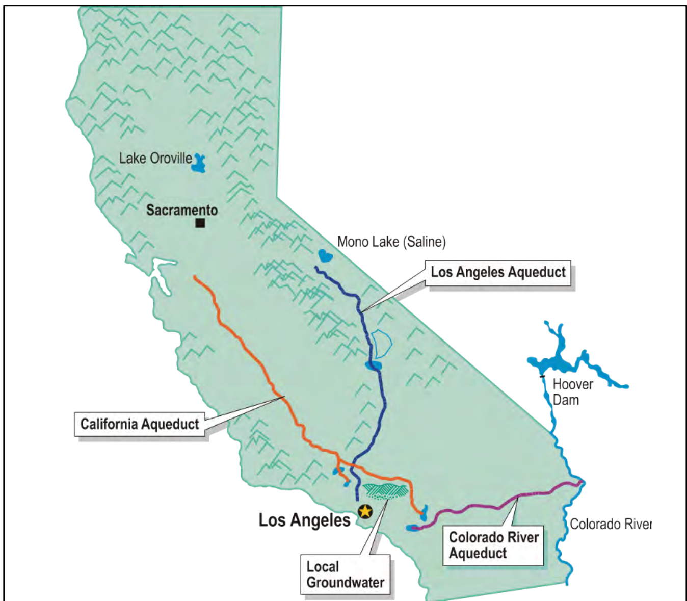
Figure 8-6. Primary Water Supply Sources for City of Los Angeles
