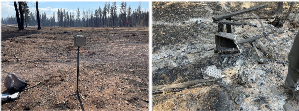
Figure 6. Left photo shows moderate to high burn severity adjacent to data logger case for soil moisture measurement in Marian Meadow. The right photo shows the remains of our sap flow instruments in Rock Creek Meadow, this was one of the few instruments that were a total loss. Photo taken one month after fire, September 2021.
