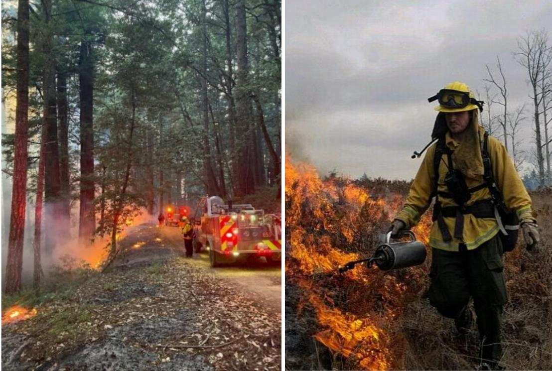
Figure 18. Examples of Prescribed Burning Equipment – Type 6 and Type 3 Fire Engines (left), Drip Torch (right)
