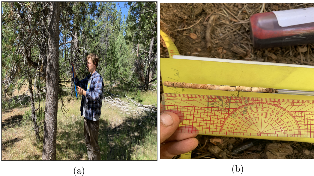
Figure 4.7: (a) Process of coring a tree with the increment borer. (b) An example tree core used to determine sapwood depth.
