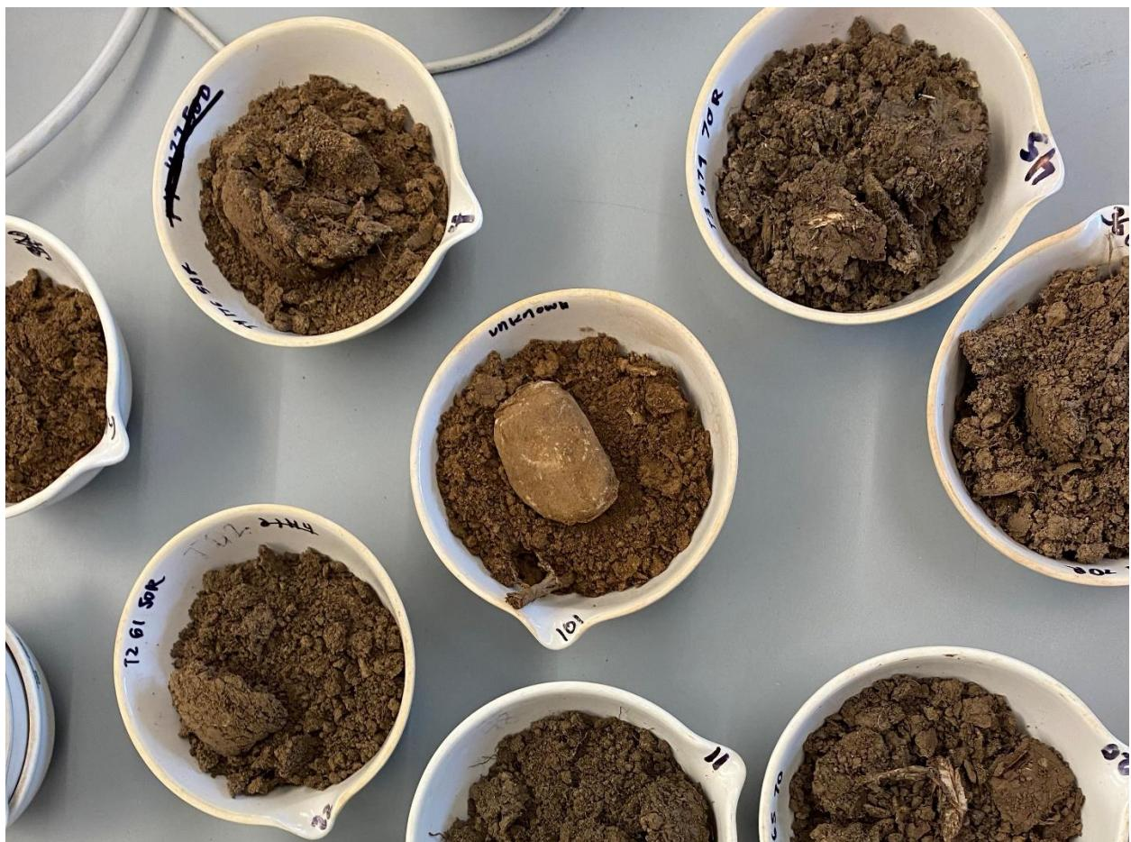
**Figure 6.** Soil bulk density sample processing. Note the large rock in the middle sample. Samples with high amounts of roots, pebbles, and rocks were not included in calculating overall soil compaction.
